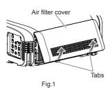
Air filter unit compartment and the projector's air intake port
